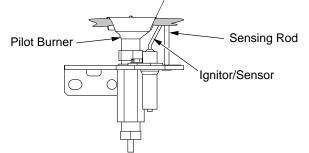
Figure 51 - Correct Pilot Flame Pattern
